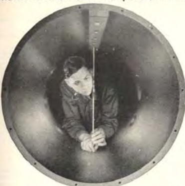
Checking Diameter of 30-Inch Cylinder Liner for Marine Diesel Engine. (Using Inside Micrometer Number 681D, built up with extension rod at both ends.)
