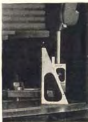
Used to Set Cutting Tool. Note Use of Extension Bar.
