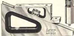
Position for Smallest Setting, \frac{1}{4} inch
