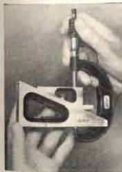
Gage Being Set to Micrometer Accuracy
